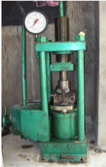
Original 51OP press on a foundation with worm attachment. Hydraulic press to the right
