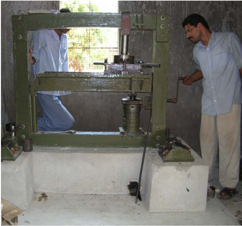
Original 51OP press on a foundation with worm attachment. Hydraulic press to the right
