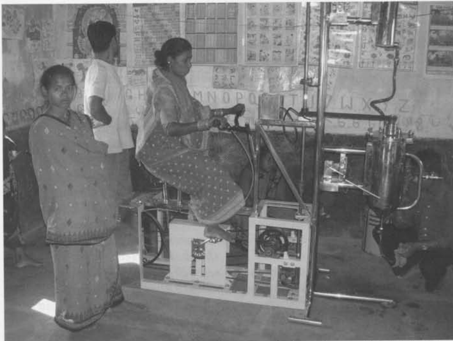
Manjula Pradhan from Kandhabanta using pedal power to mix the newly pressed oil with alcohol and lye to produce biodiesel. Sukumari, also of Kandhabanta, awaits her turn.
