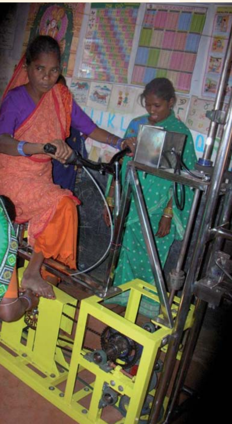
Self-Help Group women teaching each other how to pedal the biodiesel reactor at Kandhabanta-Talataila.
