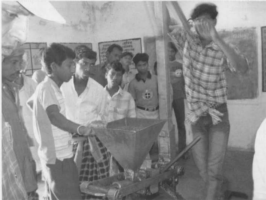
A barefoot technician trainee from Tumba demonstrating the hand-operated Mafuta Mali oil press. Niger seed grown by farmers in Tumba is being pressed during this demonstration and feedback session.
